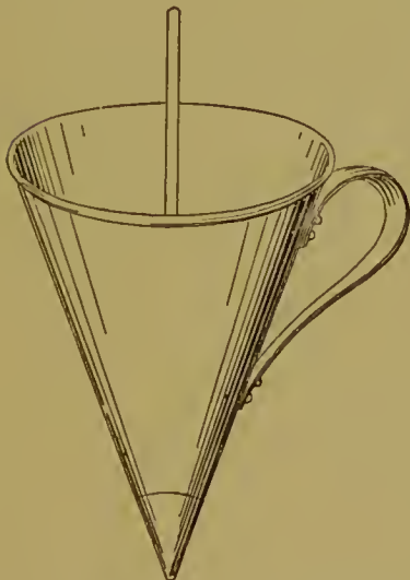
Fig. 101.—Filling Funnel for Fondants
